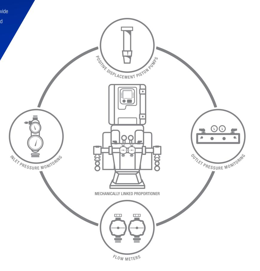
**G**raco has identified the best method of detection for issues that may cause off-ratio foam to be sprayed. These issues are called *single-point variables*. Utilizing inlet and outlet pressure monitoring and flow meters, the Reactor 2 can monitor for these issues and shut the proportioner down if required. The operator can then make the necessary updates in order to eliminate the off-ratio condition. 1
